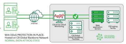
• Ingress traffic is distributed around the edge of the C8 network at a point closest to the source.
